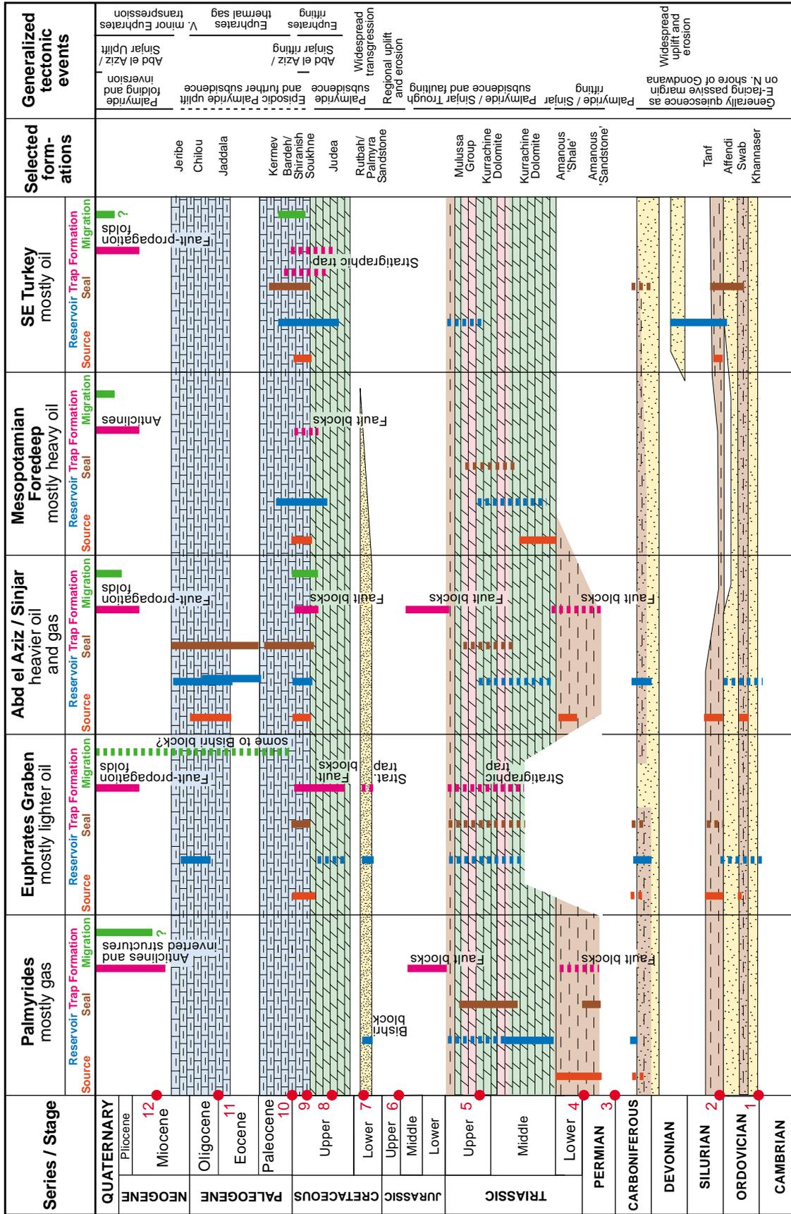
Figure 18: Generalized stratigraphy and selected structural elements in various hydrocarbon provinces of Syria and SE Turkey. Proven features related to hydrocarbon accumulation are shown as solid lines; dashed lines where uncertain. Tectonic events generalized from Figure 16. Red dots refer to time points of Figure 16. Note that formation names change between Syria and Turkey. Lithology as for Figure 9.
