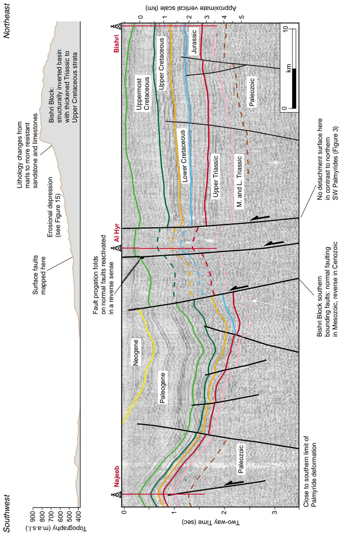
**Figure 4: Interpretation of migrated seismic profile ALAN-90-10 from SW edge of Bishri Block in the NE Palmyrides (see Figure 2 for location). Dashed interpretation is speculative because of poor data.**
