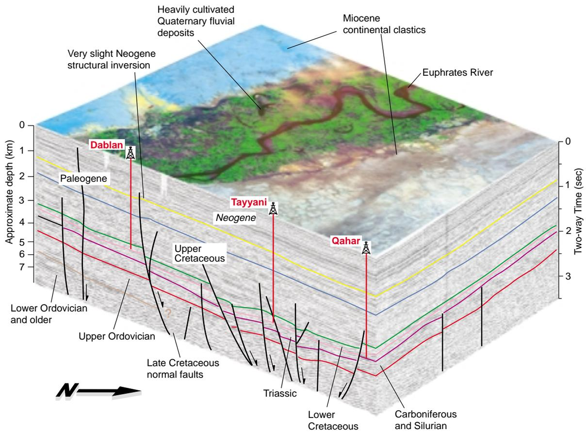
**Figure 6: Perspective block model of the Euphrates Graben (see Figure 2 for location). Surface is Thematic Mapper imagery draped over topography. Faces shown are seismic lines PS-14 (dip) and PS-11. Image 31x20 km.**
