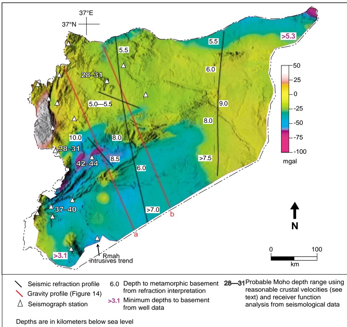
**Figure 13: Bouguer anomaly map of Syria (BEICP, 1975) together with topographic imagery. Note (1) abrupt along-strike variation in gravity anomalies in the Palmyrides coincident with topographic change, and (2) contrast between Bouguer anomalies north and south of the Palmyrides.**
