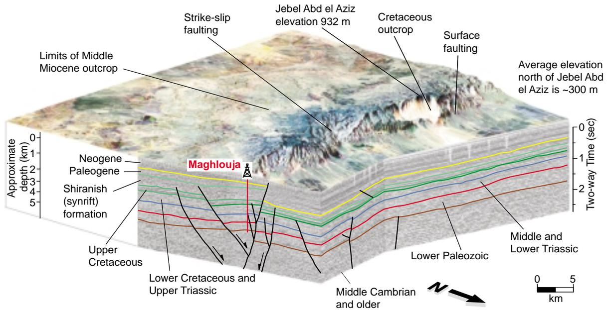
**Figure 5: Perspective block model of the Abd el Aziz uplift in NE Syria (see Figure 2 for location). Surface is Thematic Mapper imagery draped over topography. Faces shown are seismic lines UN-350 (dip) and SY-48N. Image 29x41 km: topographic exaggeration about x 5; subsurface exaggeration about x 2.**
