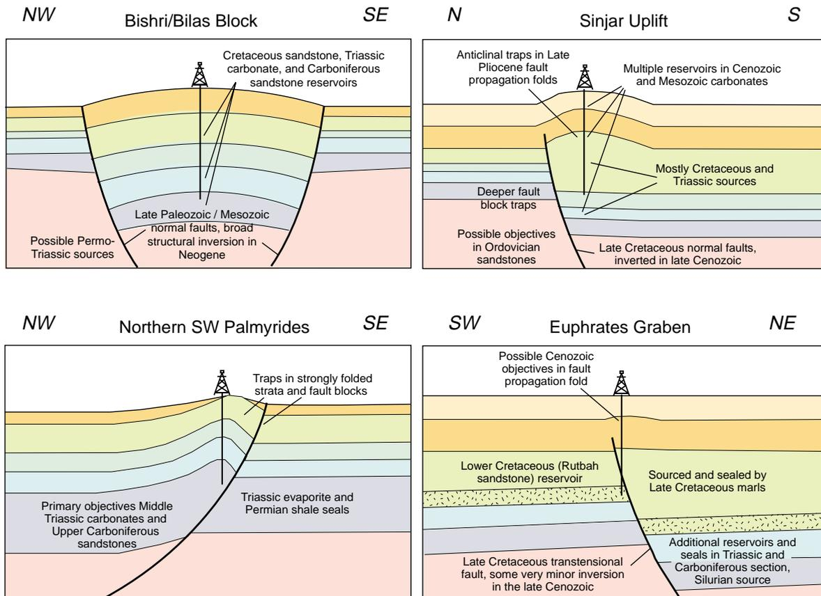
**Figure 19: Highly schematic cross-sections of examples of trapping configurations in some typical oil fields of Syria.**
