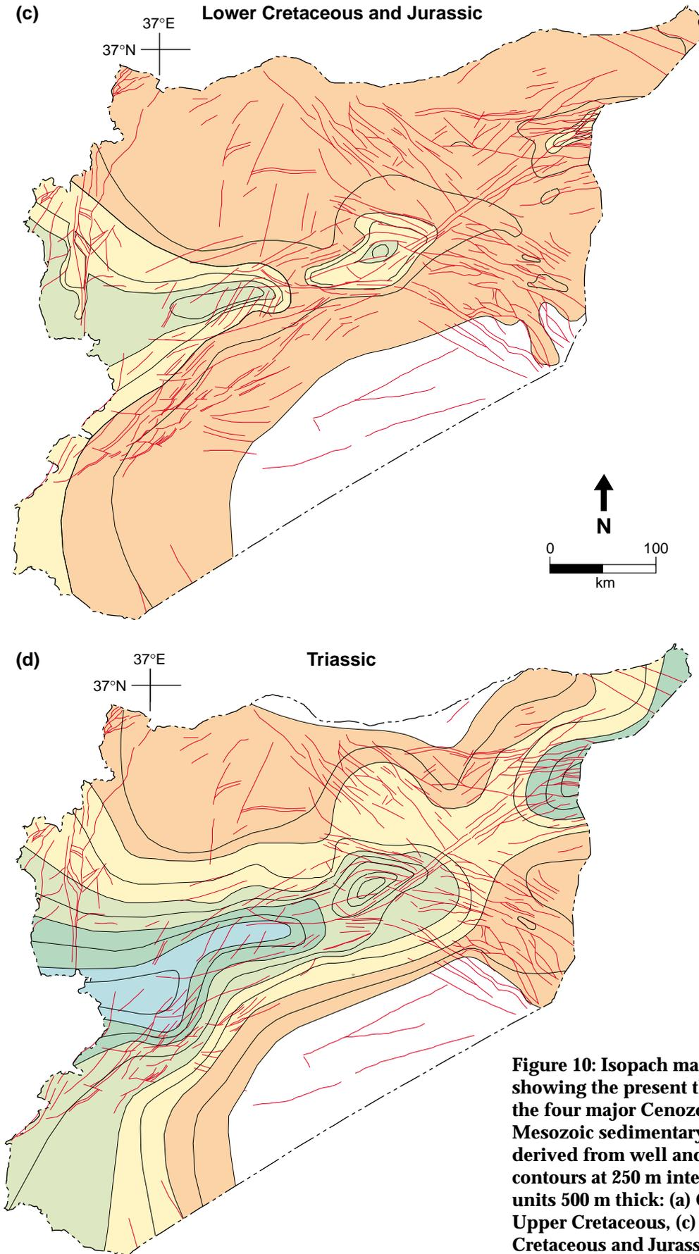
**Figure 10: Isopach maps of Syria showing the present thickness of the four major Cenozoic and Mesozoic sedimentary packages, as derived from well and seismic data; contours at 250 m intervals; colored units 500 m thick: (a) Cenozoic, (b) Upper Cretaceous, (c) Lower Cretaceous and Jurassic, (d) Triassic.**
