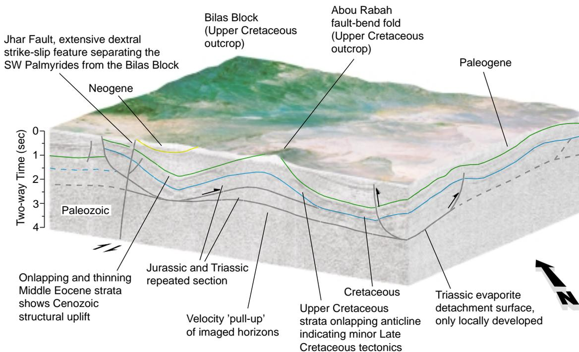
**Figure 3: Perspective block model of the Abou Rabah anticlinal structure in the northern part of the SW Palmyrides (see Figure 2 for location). Surface is Thematic Mapper imagery draped over topography. Faces shown are seismic lines CH-36 (dip line) and CH-45. Image is 31x32 km with approximately no vertical exaggeration.**
