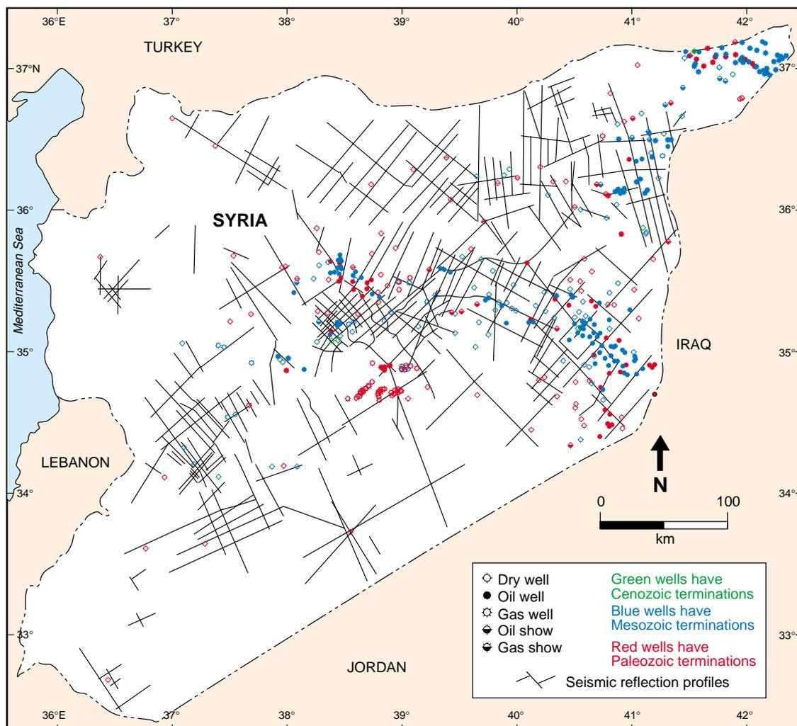
**Figure 8: Locations of seismic reflection surveys and exploration and development wells. Well colors indicate depth of penetration; symbols show best available knowledge of the status of wells summarized from various literature sources.**
