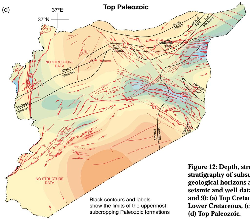
**Figure 12: Depth, structure, and stratigraphy of subsurface geological horizons as derived from seismic and well data (see Figures 8 and 9): (a) Top Cretaceous, (b) Top Lower Cretaceous, (c) Top Triassic, (d) Top Paleozoic.**
